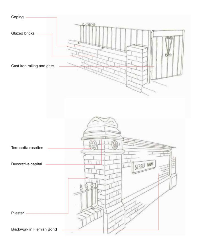
Picture 56. Front boundary wall with glazed bricks and cast iron railing
